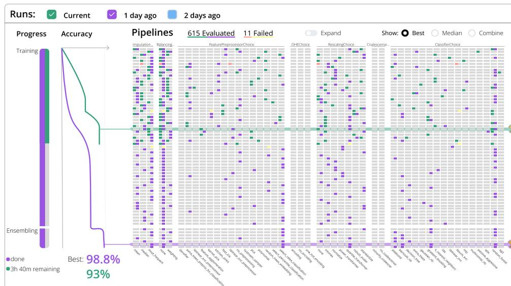
**Figure 4** Our sketched visual interface to visualize AutoML/DS systems. An ongoing Auto-sklearn optimization is visualized in green. Additional past runs can be selected at the top for comparison. The table on the right shows the best performing configurations in the specific time segment.
